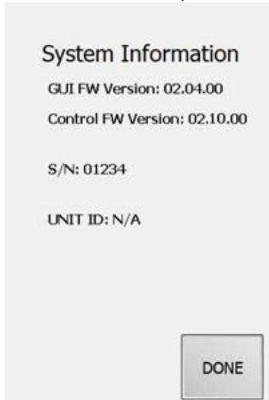
The GUI FW and Control FW version display the latest FW version on the device. The S/N is set by manufacturer during assembly and matches the control label S/N on the base of the device.
